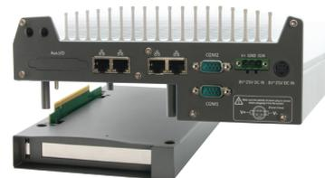
This expansion Cassette also innovates a better way of cooling for add-on cards. An optional fan is the general solution for most add-on cards. Neosys also provides shaped heat-spreaders for selected cards. As the shaped heat-spreader contacts both components and surface of Cassette, the heat generated is brought out and a stable thermal condition is maintained inside Cassette. Currently shaped heat-spreader are available for
